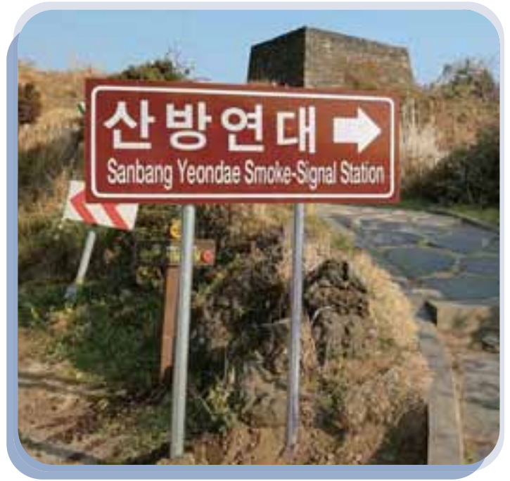
복주식 Dimension : 주문제작 Material : THK2 Aluminum Processing : sheet cutting
